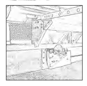
**Interior Pit Mount:** Device is recessed behind the foundation wall or part of a "deep pit" stand.
