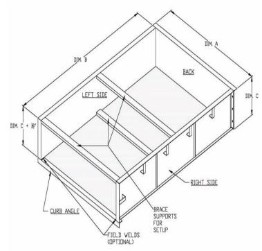
CAUTION: DO NOT USE MORE CONCRETE THAN WHAT IS NORMAL FOR PIT WALLS. DO NOT POUR CONCRETE TOO FAST OR IT MAY CAUSE BOWING IN THE PERMA PIT WALLS.
